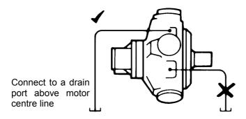
The recommended minimum pipe size for drain line lengths up to approx. 5m is  $12.0 \text{mm}^{-1}/_2$ " bore. for longer drains, increase pipe bore to keep motor casing pressure within specified limits.
