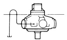
Piping (from any drain port) must be taken above level of motorcase to ensure good bearing lubrication. The arrangement must not allow syphoning from the motorcase.
