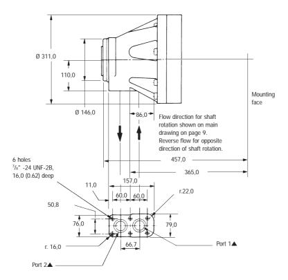
▲ Ø 35,0 with recess for 38,1 i/d x Ø 3,53 section O-ring
