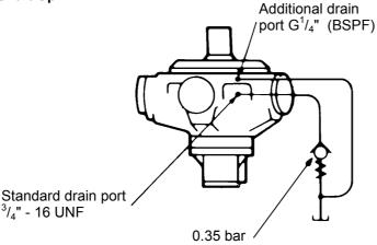
Specify "V" at model code position (3) for extra drain port, G<sup>1</sup>/<sub>4</sub>" (BSPF). Connect this port into main drain line downstream of a 0.35 bar check valve to ensure good bearing lubrication. Piping arrangement must not allow syphoning from the motor case. Where this arrangement is not practical, please consult Kawasaki.
